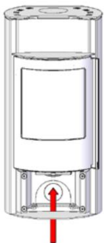
Bottom plate is prepared for combustion air.
